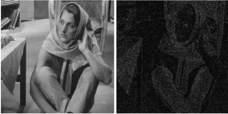
Fig. 17.6 Denoised image (i.e. fitted values) with IBR kernel ( PSNR = 33.72 dB) and image of the residuals ( right )
